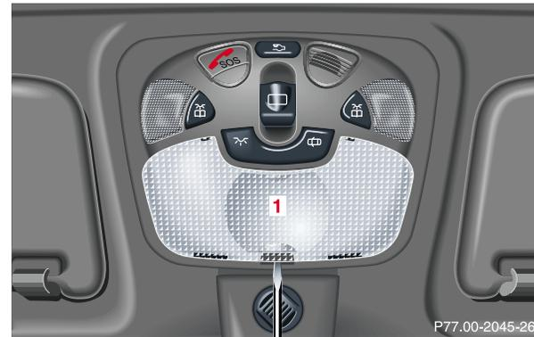
The panorama sliding/pop-up roof can be opened or closed manually should an electrical malfunction occur. The panorama sliding/pop-up roof drive is located behind the lens (1) of the interior overhead light. Pry off the lens (1) using a screwdriver.
