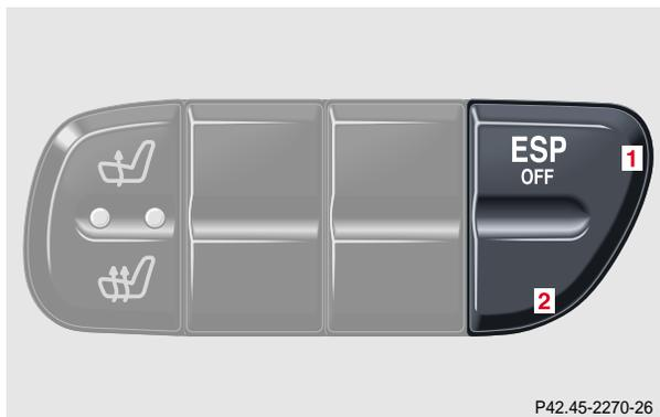
ESP control switch located on center console.
