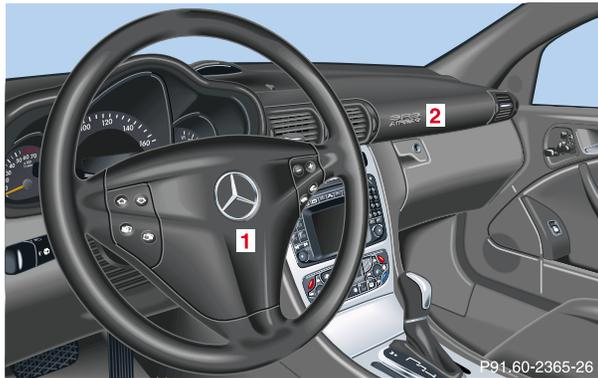
**1** Driver airbag**2** Front passenger airbag
